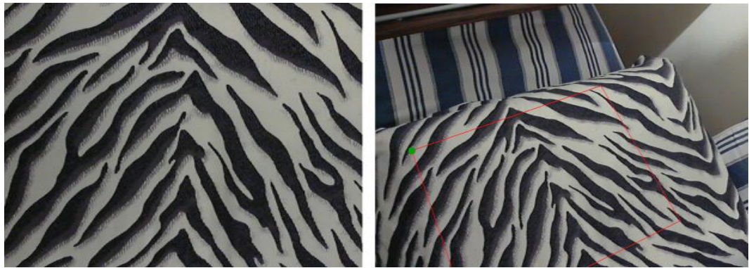
Figure 7.4: A sample result of SIFT tracking. The selected pattern was found on the real-time image in average 117ms.
