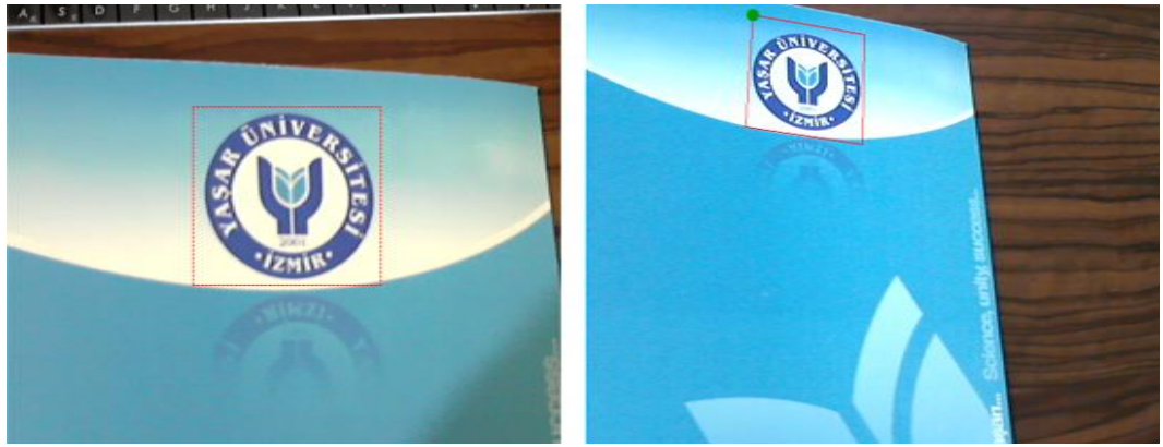
Figure 7.3: A sample result of SIFT tracking. The selected area was found on the real-time image in average 78ms.
