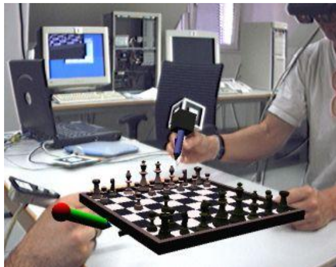
Figure 2.6: A game of AR Chess demonstrates collaboration of the stationary user (left) and the mobile user (right) as seen by the "documentation camera" user.
