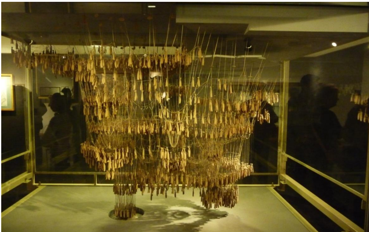
Figure 5. Gaudi's String Model with Birdshot Weights Used in the Design of the Colonia Guell (Asmaljee, 2013)
