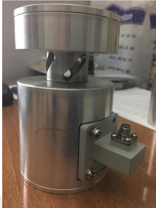
Figure 46. Fabricated Receiver Antenna.
