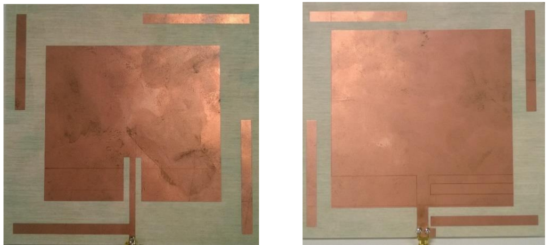
Figure 6.9 The front and back view of produced linearly polarized UHF RFID reader antenna
