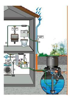
Roof rain water in the buildings are filtered and sent to pure water store. This water is used for watering the garden or fire extinction and it can be softened to be used as campus use water (Figure 4.10.).
