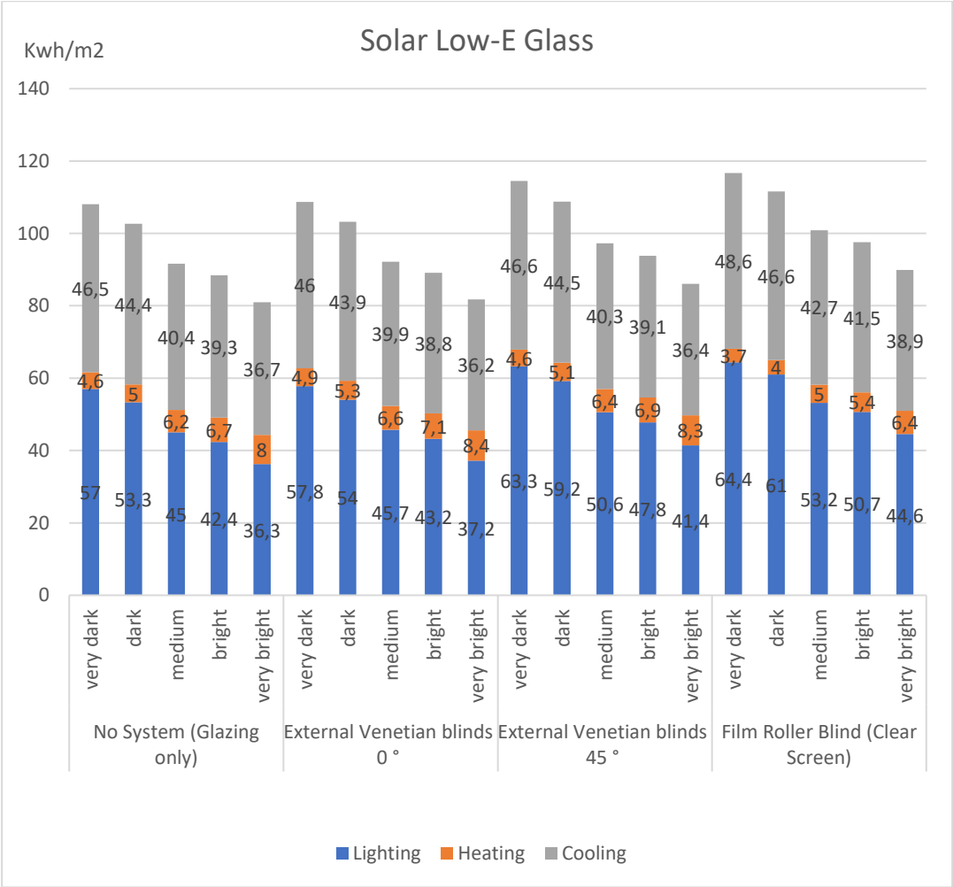
Figure 5. 6. In the use of Solar Low-E Glass According to Reflection values Annual Energy Consumption Lighting (L), Heating (H), Cooling (C)
