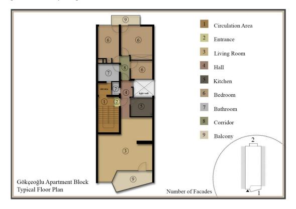
**Figure 4.15.** Gökçeoğlu Apartment Block floor plan and functions. Drawn and produced by the author.
