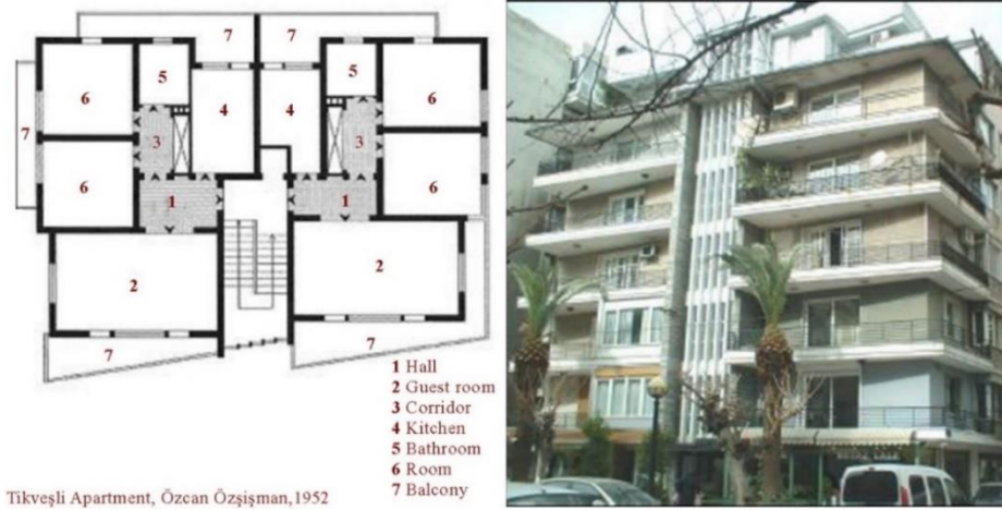
Figure 3.11. Tikveşli Apartment, Alsancak, Özcan Özşişman, 1952, plan and street view (Ballice, 2006, 175, marked by the author)
