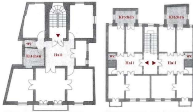
Figure 3.7. Sofas turned into access halls in apartments of the 1930s (Gökmen, 2011, 14, marked by the author)
