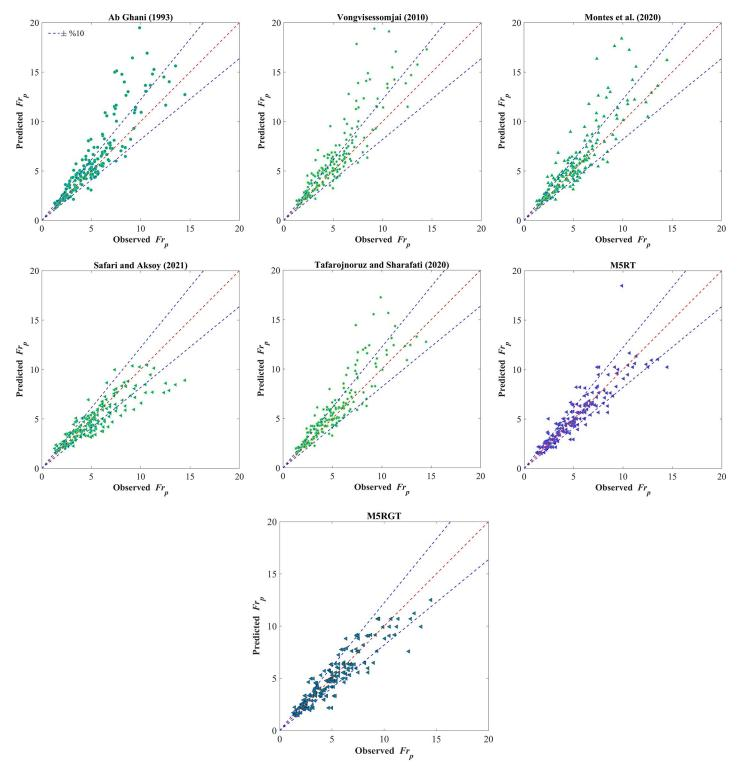
Fig 3. Scatter plots for observed and predicted particle Froude numbers for the testing stage.
