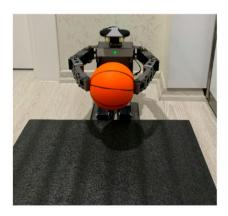
Figure 7. The Robotis-Op3 humanoid robot and its object manipulation photo.
