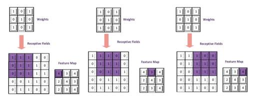
Figure 2. The results of the convolution processes for one depth channel of the image.
