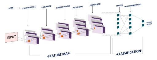
Figure 1. An CNN structure and the layer representation.
