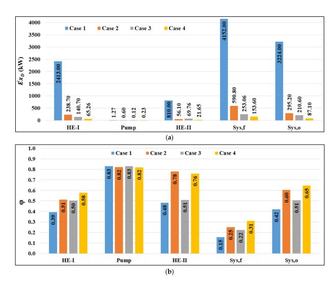
Figure 4. Conventional exergy assessment results based on (a) exergy destruction rate and (b) exergy efficiency.
