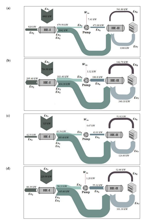
Figure 3. Grassmann (exergy flow) diagram of the created cases, (a) case one, (b) case two, (c) case three and (d) case four.
