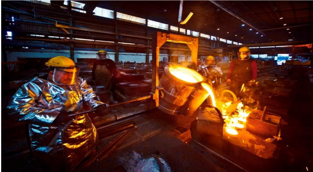
Figure 3.4. Pouring molten metal into the sand molds Photo is taken by Sezgi ÇELİK
