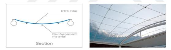
*Figure 29: Single layered ETFE* Source: (Sert, 2016)
