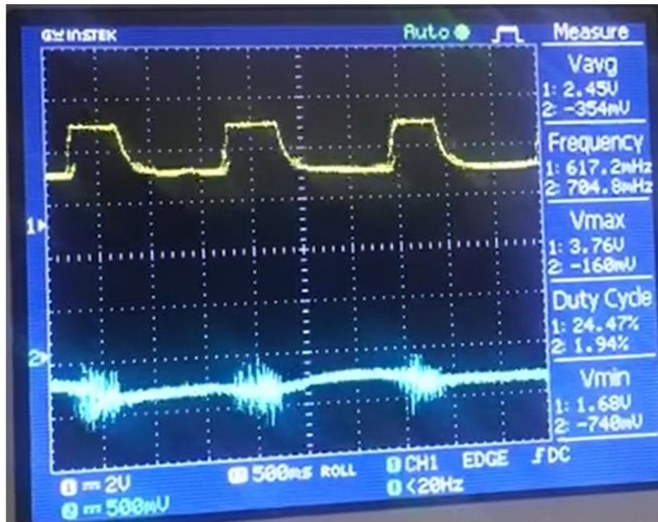
Figure 3. 22 Oscilloscope image of the EMG kit output and raw EMG signal.
