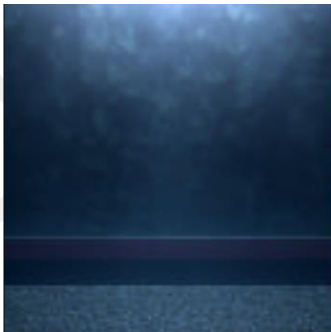
Figure 4.6. Cerezo & Seron's (2002) study of simulating sea water with very low phytoplankton abundance. The change in the color is a result of chlorophyll concentration which starts to move to green from blue in certain pixels (in the shifted part, the color becomes lighter as a result). The discrete ordinates method was used in the solution of RTE.
