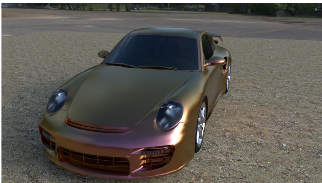
Figure 7.7. A car object rendered with a coating of translucent flakes (80 nm \text{TiO}_2 – 80 nm \text{SiO}_2 – 80 nm \text{TiO}_2 )
