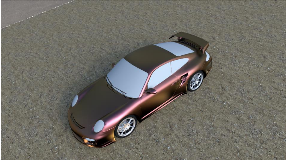
Figure 7.18. The Micro-Flake model using a composition of 80 nm \text{TiO}_2 translucent flakes modelled on a car object. In the scene, the color shifts are observed and they are accurate with the results shown in the chapter 6.
