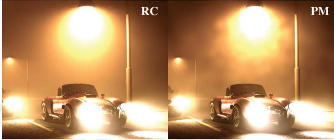
Figure 4.5. A sample scene comparison rendered with Jarosz et al.'s (2008) radiance caching method (left) and traditional photon mapping (right). The quality is better in the proposed method which combines the stored sample information with the gradient information.
