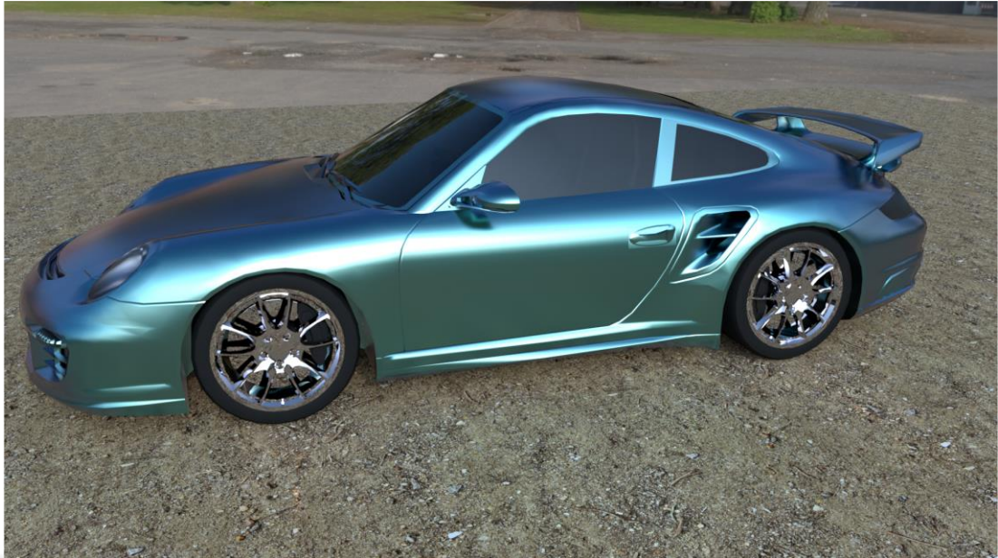
Figure 2.5. Ergun et al.'s rendering of car paint material composed of translucent flakes. (Ergun et al., 2016)
