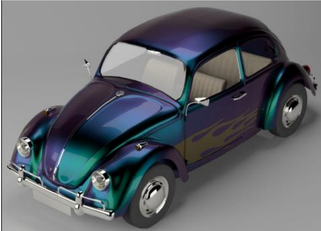
Figure 2.6. An example scene of Belcour and Barla’s study. The researchers rendered color shifts in car paints. However, sparkles were not represented in their model (Belcour & Barla, 2017).
