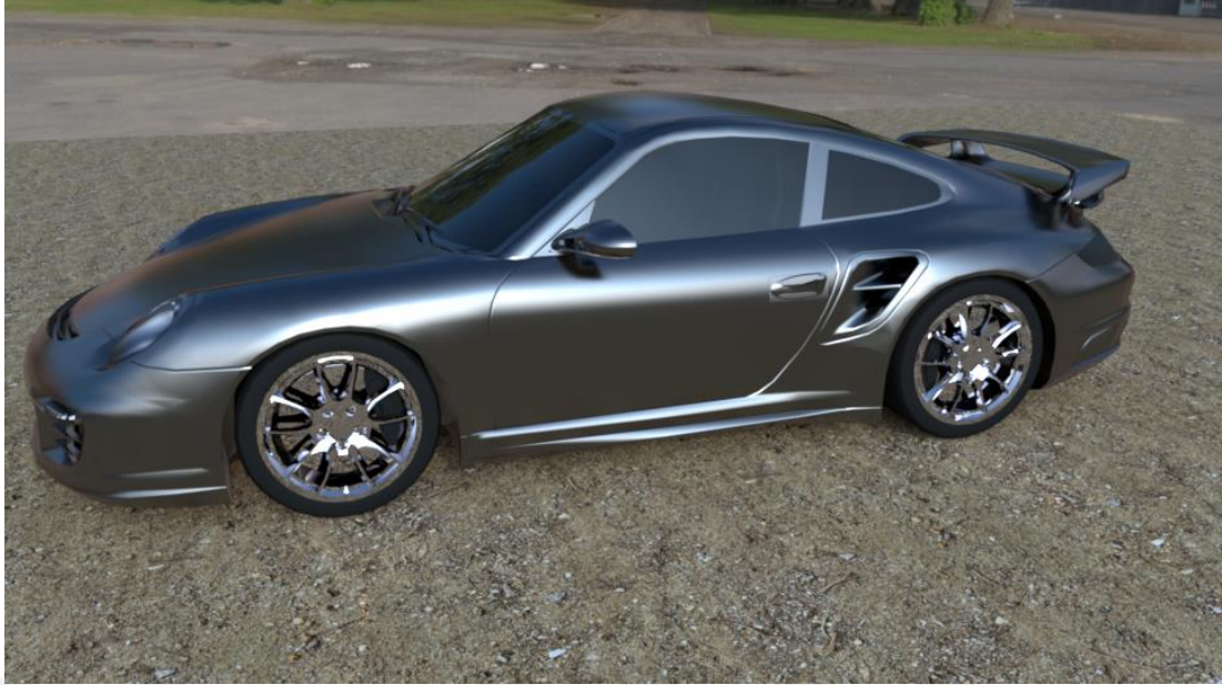
Figure 7.8. A car object rendered with a coating of translucent flakes (80 nm \text{TiO}_2 – 80 nm \text{SiO}_2 – 80 nm \text{TiO}_2 )
