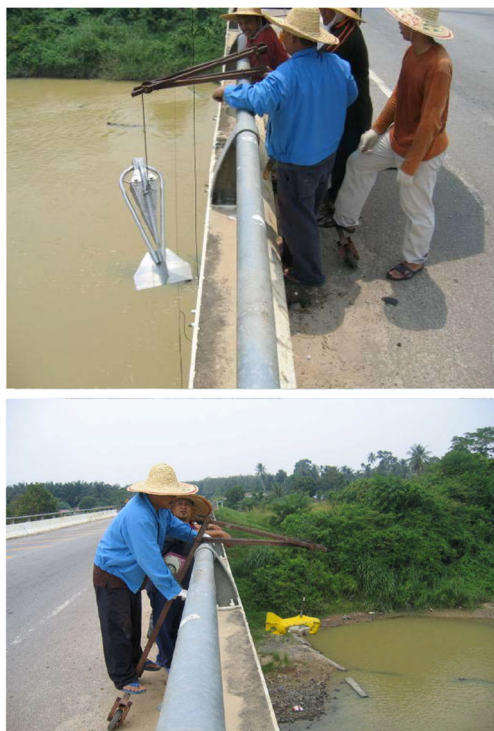
Fig. 5 Data collection of bed load and suspended load by using suspension from the bridge
