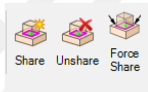
Figure A1.34. Share topology in geometry component is simply processed by 'Share' button on the ribbon.
