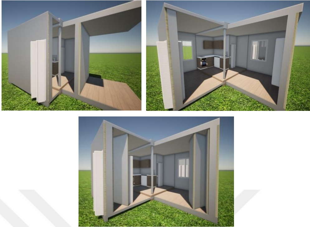
Figure 4.12. Opening Stages of the Unit
