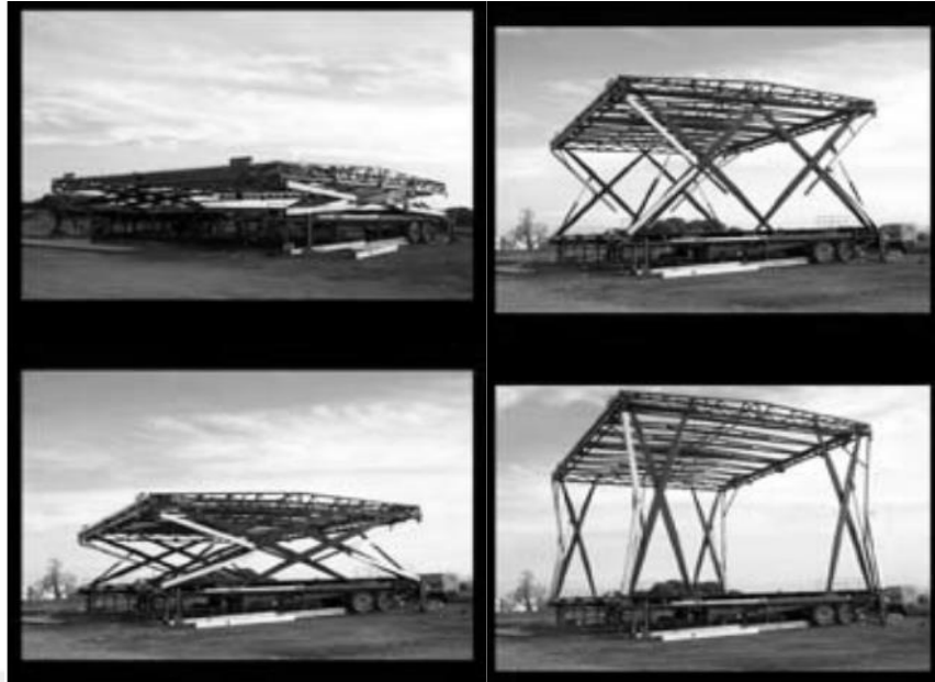
Figure 2.7. Deployment Stages of the Twinstage
