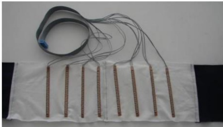
Figure 5. Wireless sensor belt to monitor foetal movement (Borges, 2010).
