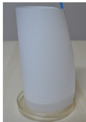
Fig. 10 Impregnation of \text{AgNO}_3 concentration on chromatography paper in the rising picture method
