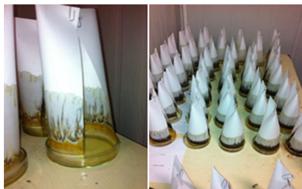
Fig. 11 Impregnation of \text{FeSO}_4 concentration on chromatography paper in the rising picture method
