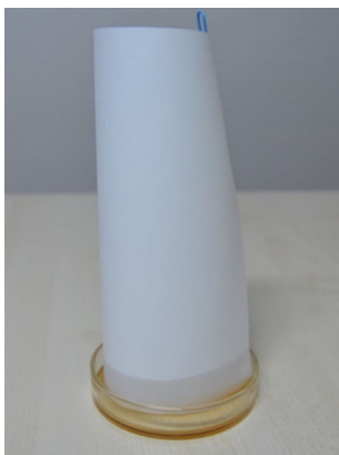
Fig. 9 Impregnation of sample concentration on chromatography paper in the rising picture method
