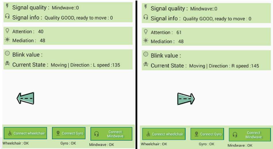
Figure 5.25 Wheelchair moving left/right directions
