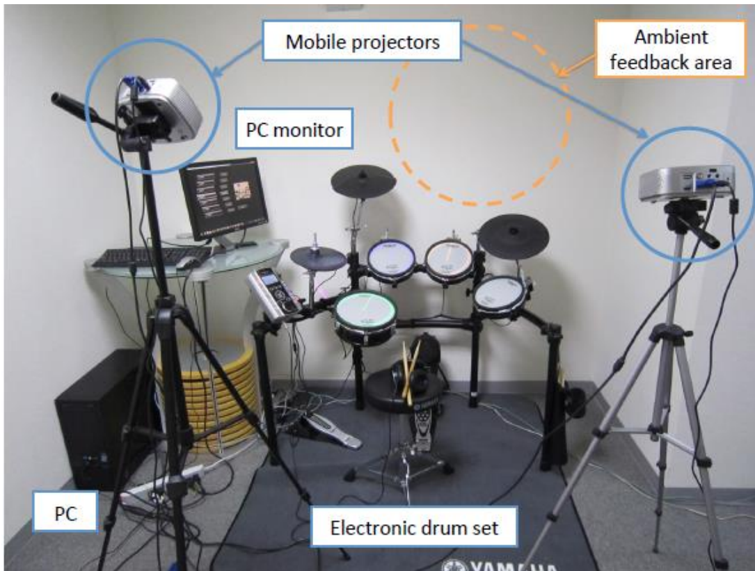
Figure 11. The setup of the AR Drum Kit by Waseda University (Yamabe, Asuma, Kiyono, & Nakajima, 2011)
