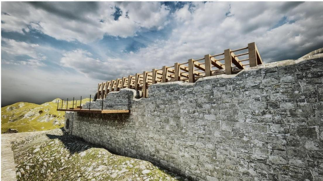
**Figure 4.13.** The steel balcony extension on the north wall of the inner castle and the pergola legs placed on the wall.
