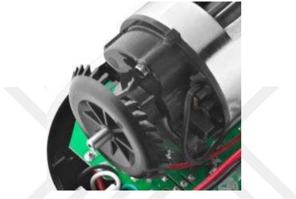
Figure 3.3. Inside view of the dc motor used in the KitchenAid
